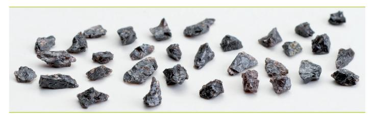
BROWN FUSED ALUMINA FESI is a non-disposable abrasive based on aluminium oxide and ferrosilicon. The product meets the requirements in accordance with BGR 500, part 2, chapter 2.24, "Working with blasting equipment (blasting work)".
